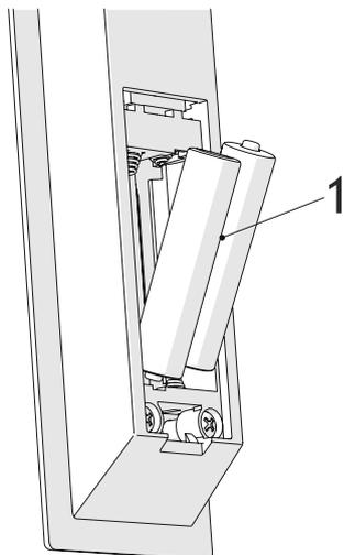
There are two batteries in your remote control. Pull the batteries by pressing + poles and remove from the battery slot (Fig. 22).
