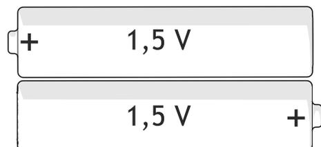
Fig. 23: **REMOTE CONTROL BATTERY PLACEMENT**
